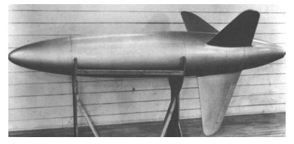
The JB-3 had an ellipsoidal, streamlined body with three wings placed 120 degrees apart. It was powered by two solid fuel rocket motors: one to accelerate the missile to 600 mph, and the other to maintain its speed over the missile's 5-9 mile range. The 100-Ib warhead could be exploded by either a proximity fuse, which was part of the radar homer, or by impact. Ramo accepted the position and started work in October of that year.
