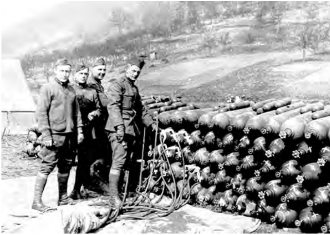
"Four soldiers with either the 1st or 2nd Balloon Company posing next to hydrogen gas cylinders with manifold and tube." (Image from The University of Tulsa, McFarlin Library, Department of Special Collections & University Archives , image 2001.073.1.016.)
