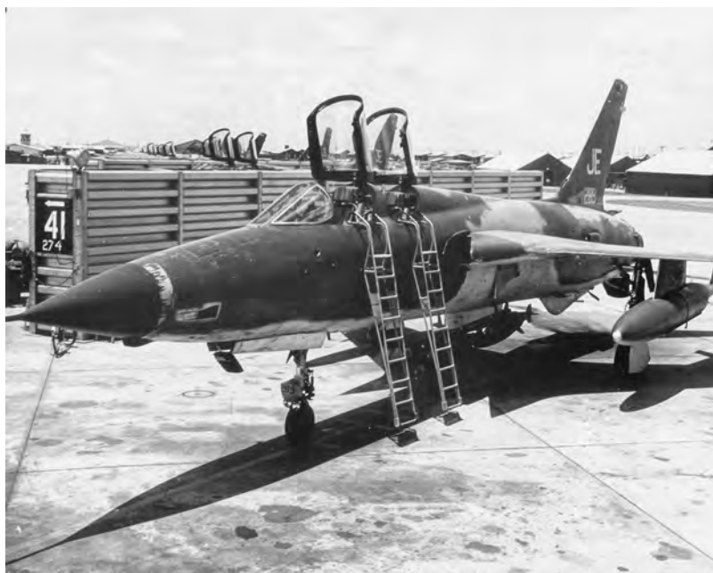
F-105F 63-8289 was one of the six 2098-modified Commando Nail aircraft in the 44 TFS. Without Azimuth-Elevation antennas, it did not have Wild Weasel equipment and lacked a control stick in the rear cockpit. It was lost on Sept. 7, 1968 due to engine failure. Its crew, Maj. Eugene A. Bonfiglio and EWO Maj. Lorne F. McCormick, ejected successfully with minor injuries.
