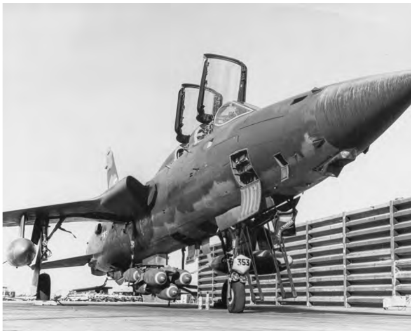
With its triangular, SAM-locating Azimuth-Elevation antennas aft of the radome, F-105F 63-8353 was one of the planes in the 44 TFS with dual capability for Wild Weasel and Commando Nail missions. It was lost to AAA during a Wild Weasel mission in Route Pack 1 on July 15, 1968. Its pilot, Maj. Gobel D. James, became a POW and its EWO, Capt. Larry E. Martin, was killed.
