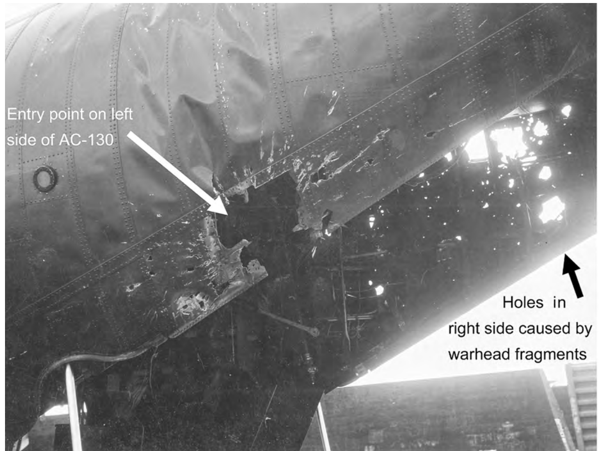
(Above right) Photograph of the damage the SA-7 caused to Felty's AC-130. (Below) Felty's helmet.
