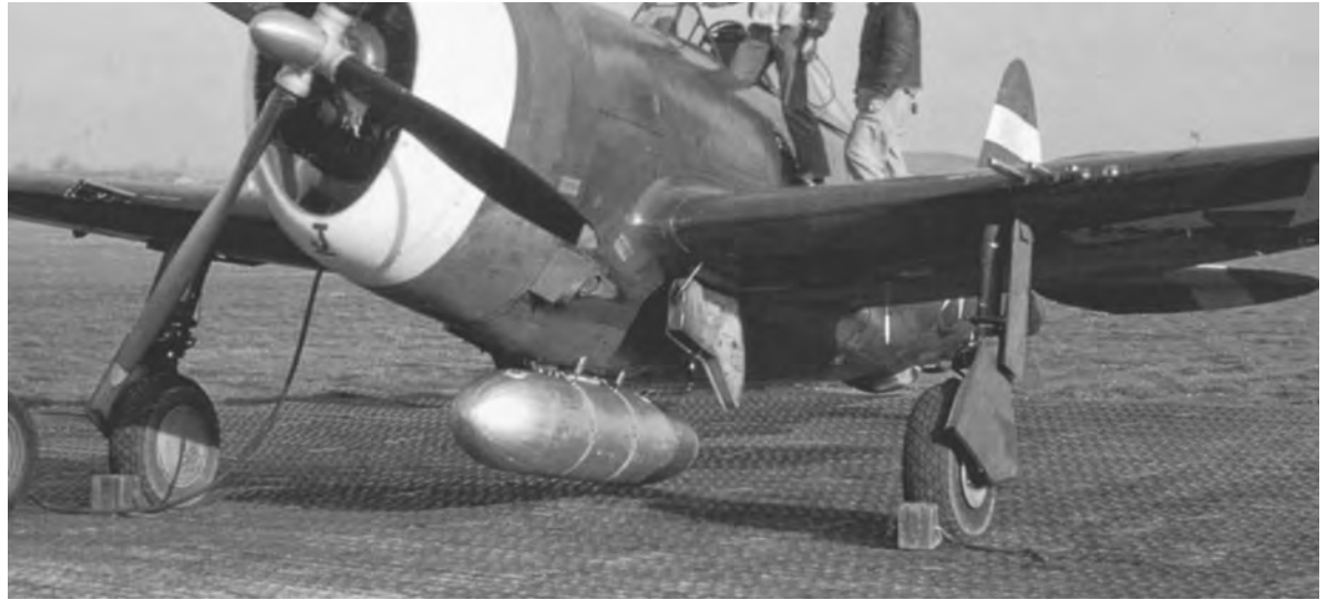
A P-47 in England in late 1943. Note how close the centerline external tank is to the ground.
