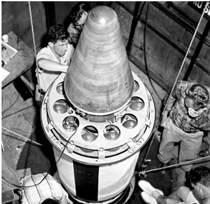
Figure 12: Jupiter-C sub-scale reentry vehicle attached to the spinning “tub.” This vehicle was an early fiberglass-melamine ablative material flown on 15 May 1957. While not recovered, the telemetry showed that the ablative concept worked well on an IRBM trajectory. (NASA photograph courtesy of Joel Powell.)
