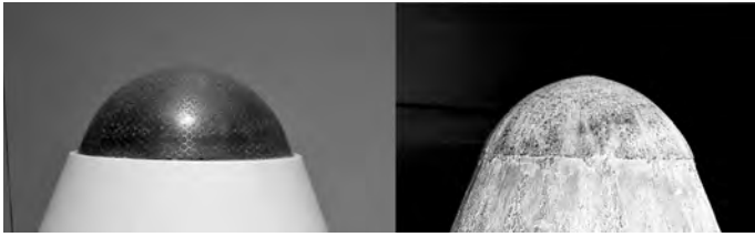
Figure 22 The effect of reentry on the Avcoite nose cap material of a Mark 5 reentry vehicle, left and right, before and after respectively. The modified Avcoite ceramic material did not melt and flow as much as on the Mark 4 (photographs by author of artifacts at the National Atomic Museum).
