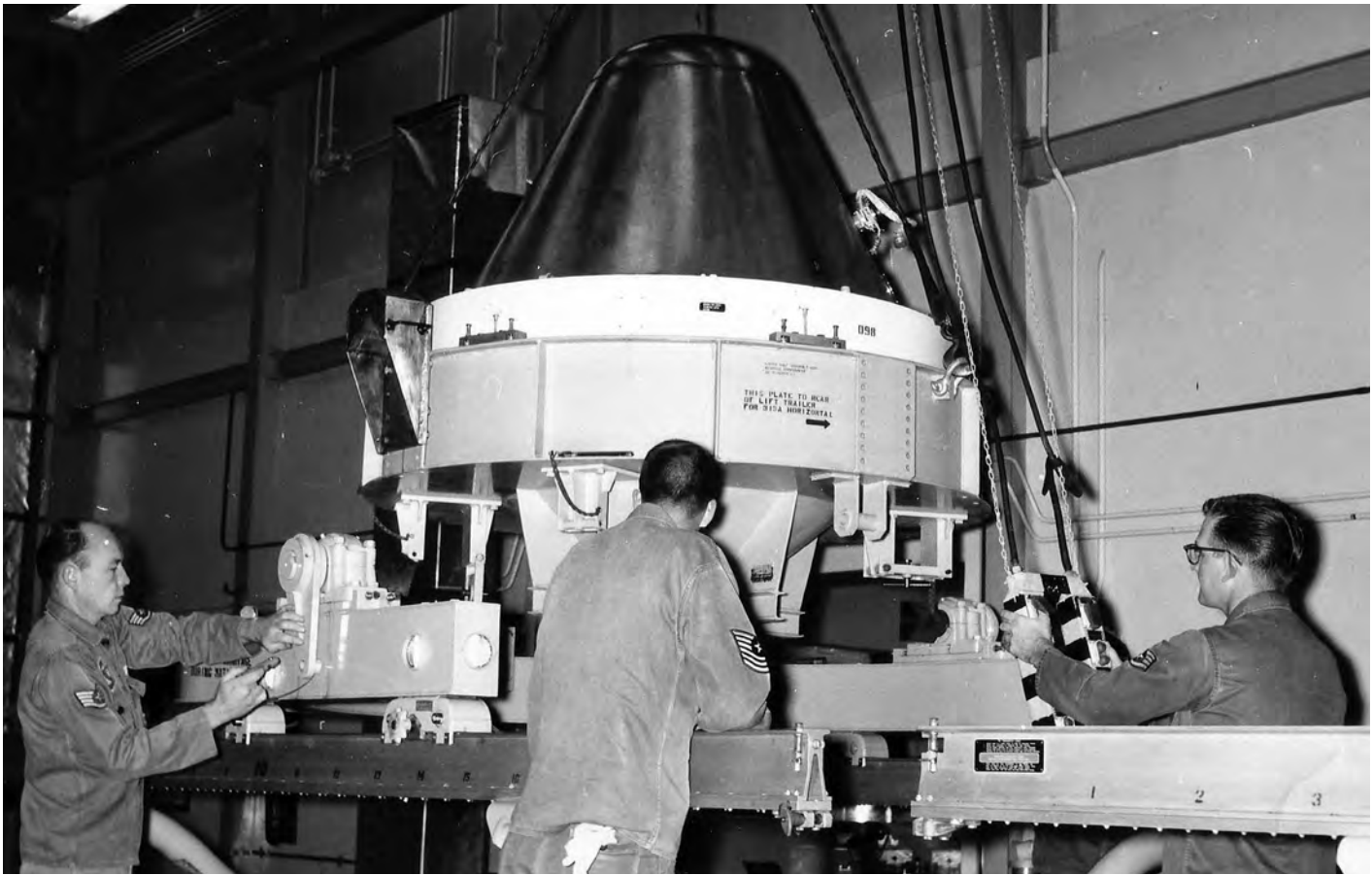
Figure 11: Mark 2 reentry vehicle (shown upside down) being inspected prior to loading on a Thor missile in England. (Courtesy of Jim Causby)
