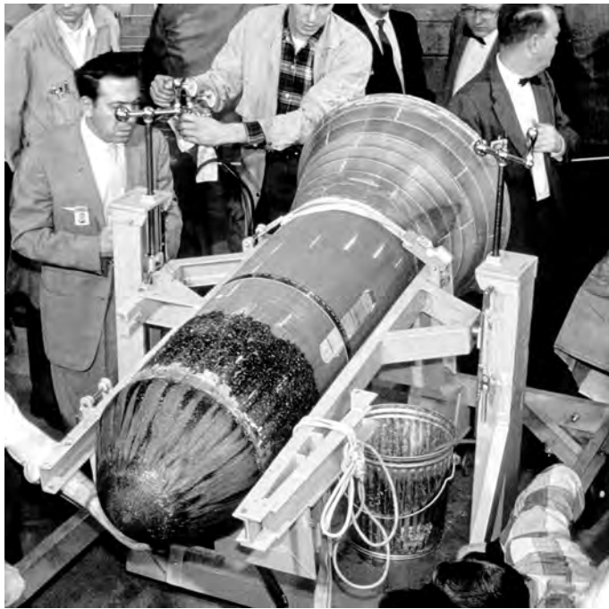
Figure 17: The Avco RVX – 1, launched on 8 April 1959 on Thor missile 133, was the first recovered reentry vehicle flown on an ICBM trajectory. Before being put on display to the press the original nose cap was removed and replaced with a mockup for security reasons. This artifact was given to the Smithsonian Institute and is in storage at the National Air and Space Museum (photograph courtesy of Phil Fote).
