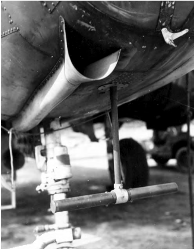
Detail shot of the direction finding antenna fitted to B-25J s/n 43-27983 'Beautiful Ohio' of the 42nd BG (M). Once an RCM observer like Lt Alderman had a fix on a site, the pilot could fly over the radar and either take photographs or attack the installation. (James Alderman via Jim Alderman)
