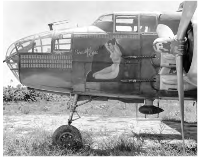
42nd Bomb Group (M) B-25J s/n 43-27983 'Beautiful Ohio' was converted to a radar-hunting ferret by Field Unit 13 personnel in October 1944. This photo was likely taken in September 1945 at Palawan's Puerto Princessa airfield. (Air Force Historical Research Agency)
