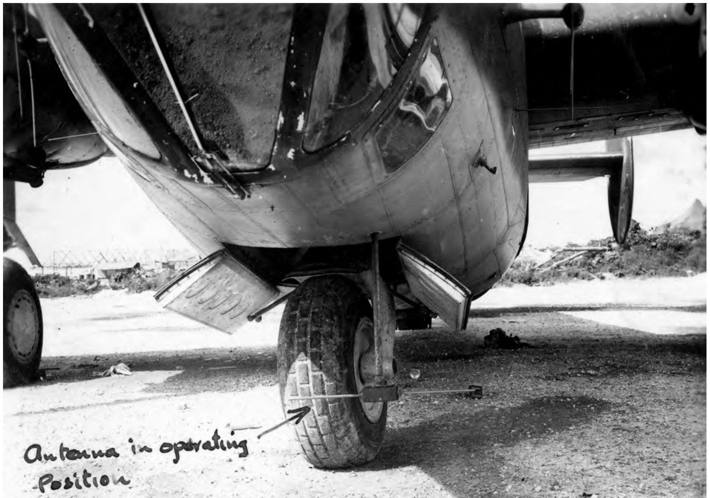
Detail shot of the direction finding antenna fitted to an early 868th Bomb Squadron B-24 'ad-hoc' ferret, Noemfoor, December 1944. (AG-989; Hocken Collections, University of Otago, Dunedin, NZ)
