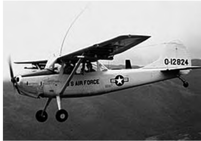
One of the main aircraft flown by Forward Air Controllers the Cessna O-1 Bird Dog.
