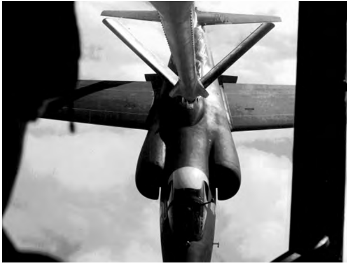
A U-2F refueling as seen from the refueling boom operator's position. The U-2F was a refuellable U-2C while the U-2E aircraft that deployed in 1964 was a U-2A aircraft modified for inflight refueling. (Photo courtesy of Chris Pocock.)
