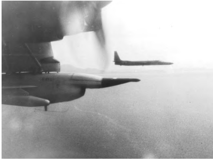
Ryan Model 147SDL being carried on the wing of a DC-130 in flight as viewed from the cockpit of the DC-130. A U-2R flies in formation off the port wing of the DC-130 to show the reconnaissance airframes associated with the 100th SRW. Circa 1972-74
