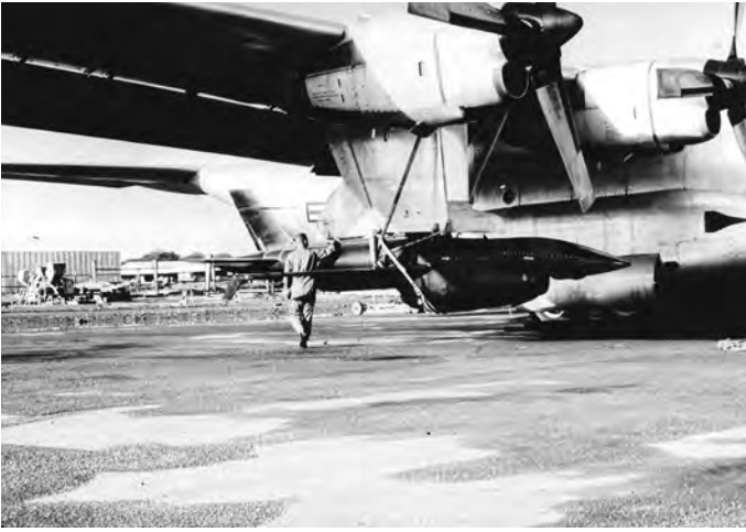
A dark painted Ryan Model 147J mounted on the wing of a DC-130 at Bien Hoa AB, RVN, April 1966, the same month the Model 147J model, a 147G model optimized for low altitude work, started operations in SEA. Between April 1966 and November 1967 the Model 147J flew 94 sorties with a 65 percent recovery rate.
