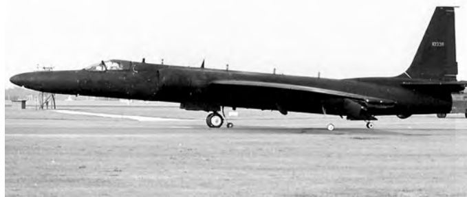
U-2R fitted with SENIOR BOOK SIGINT payload as seen in the UK, circa late 1970s. The SENIOR BOOK payload used the Melpar HARC II sensor controlled by a ground station at Nakhon Phanom Royal Thai Air Force Base to provide COMINT collection over Laos and the Gulf of Tonkin. (Photo courtesy of Chris Pocock.)
