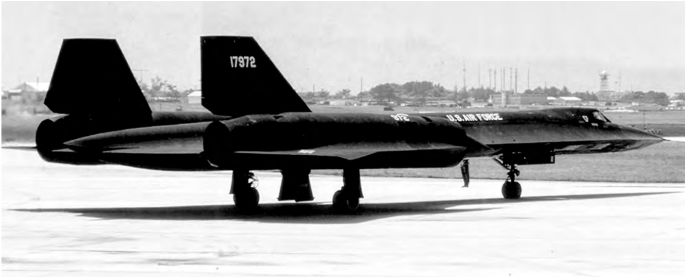
The Lockheed SR-71A offered a good platform but its sensors initially limited its utility. Even after receiving better optical cameras, it was essentially limited to cloud-free days as its all weather radar imagery payload had poor resolution. This SR-71 is depicted post-war, possibly at RAF Mildenhall, UK.
