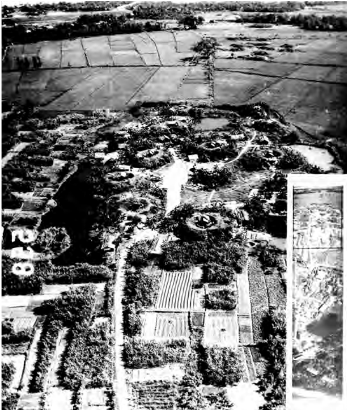
Imagery from a Ryan 147S/AQM-34L operational mission flown over the DRV on October 6, 1968. The Model 147S took horizon to horizon imagery, which is a strip at lower right; the main photo is an enlargement of the top third of the image strip depicting a DRV AAA site disguised to look like an SA-2 site
