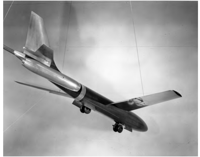
CL-52 Model during wind tunnel test in 1956 at the Canadair Plant. (Photo courtesy of Bill Upton.)
