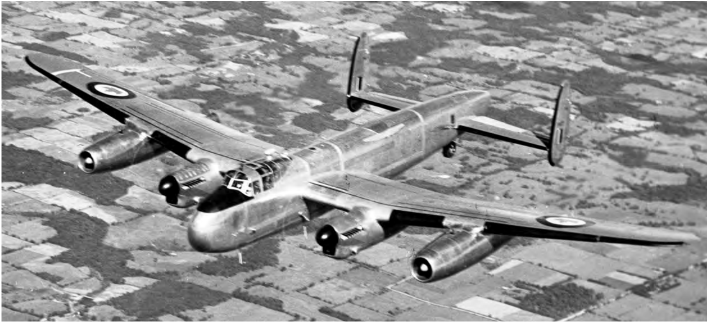
Avro Lancaster Mk 100 (Tail #FM209) which served as the testbed for the Orenda 11 engines used in the CF-100. (Photo courtesy of the Canadian Warplane Heritage Museum.)
