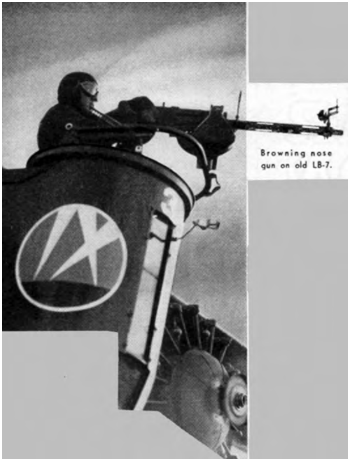
LB-7 single forward gun mount, 9th Bomb Squadron. (Photo courtesy of the Margaret R. Gundy Memorial Library, Bristol, Pennsylvania.)
