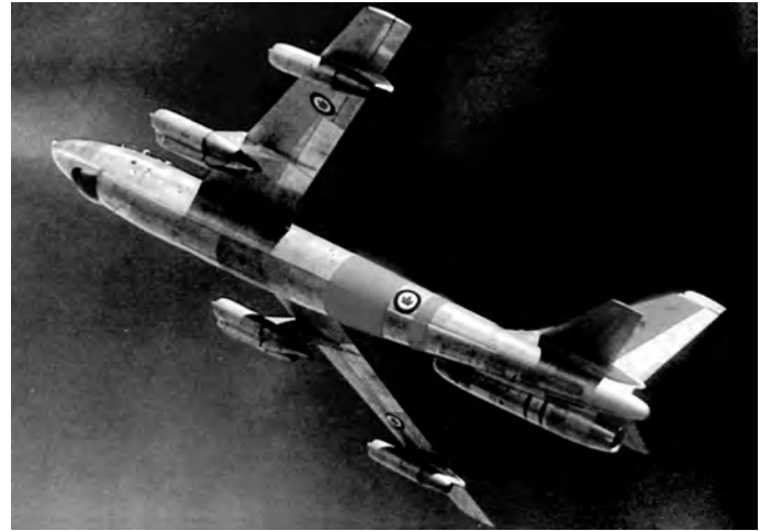
RCAF CL-52 X059 during a test flight with the Iroquois engine mounted. (Photo courtesy of the Office of Royal Canadian Air Force History and Heritage.)
