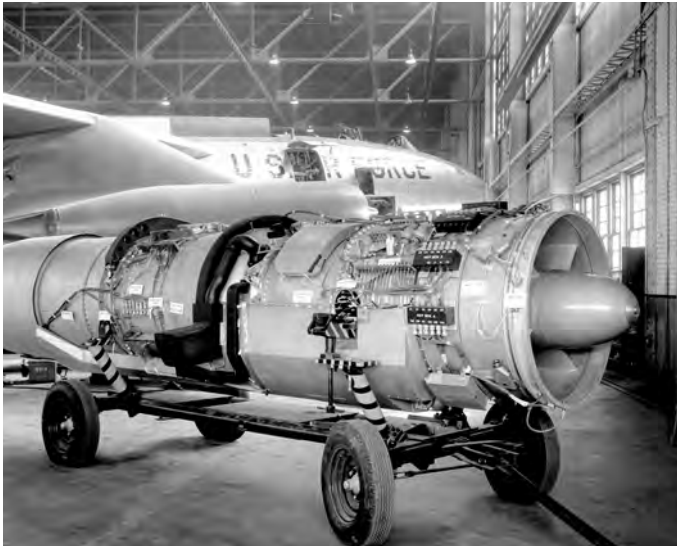
Iroquois Engine mock-up prior to mounting on the CL-52 at the Canadair Plant, Cartierville, Quebec, Canada. (Photo courtesy of the Office of Royal Canadian Air Force History and Heritage.)
