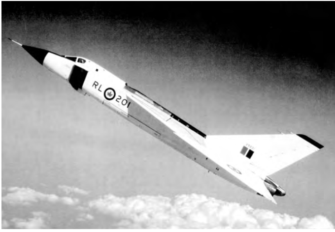
Avro Arrow 201 during a test flight with the US designed Pratt and Whitney J-75 engine while the Orenda Iroquois was in development. (Photo courtesy of the Edenvale Aviation Heritage Foundation Museum.)
