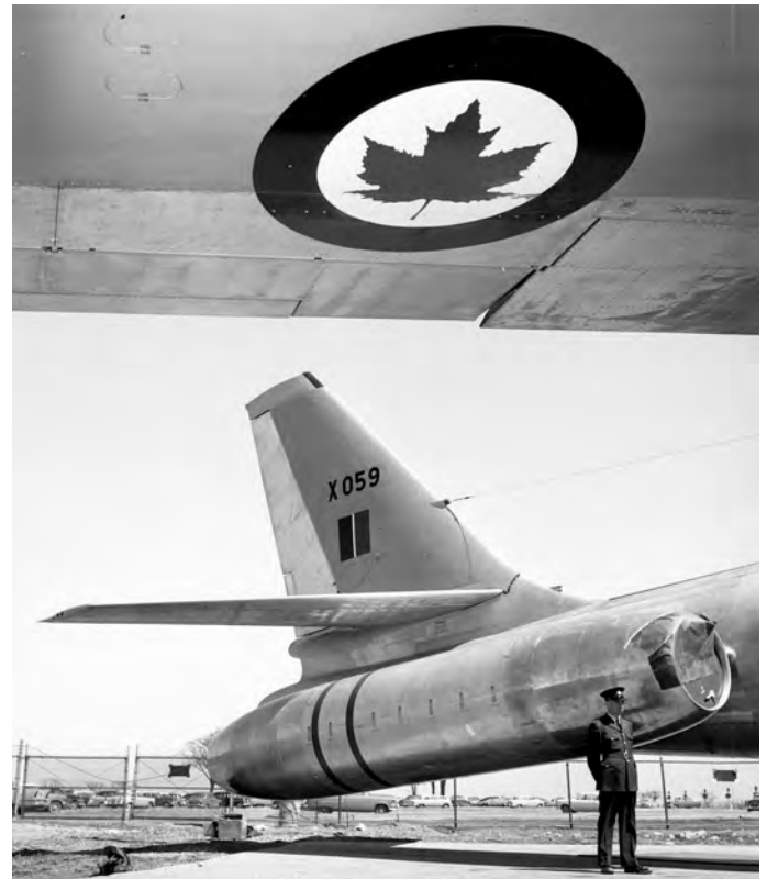
Orenda Iroquois Engine Mounted on the CL-52. (Photo courtesy of the Canadian Air and Space Museum.)
