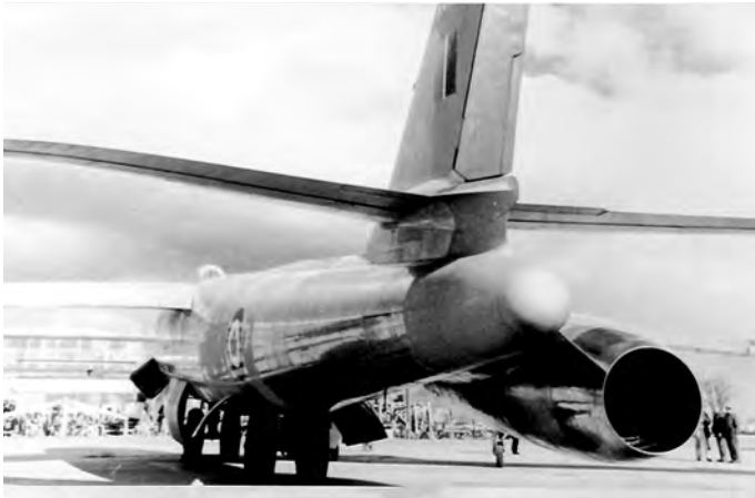
The RCAF CL-52 X059 during ground tests of the Orenda Iroquois engine. (Photo courtesy of the Office of Royal Canadian Air Force History and Heritage.)
