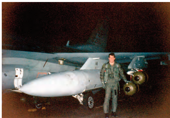
In general one nighttime and two daylight packages were flown from the Lik each day. The photo shows a 23rd TFS pilot standing in front of his Block 30 F-16C, 86-0260, prior to a nighttime combat sortie. The aircraft is configured with CBU-87s and a centerline ECM pod. (Karl Dittmer)
