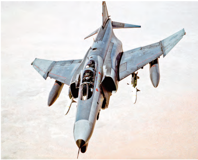
The crew of this 561st TFS F-4G is banking away from the KC-135 they refueled from. The refueling port, located behind the cockpit, is still open. The aircraft is configured with at least two fuel tanks on the outboards and two HARMs on the inboards. (USAF)
