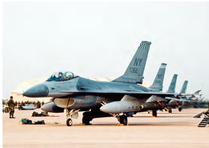
F-16As of the Air National Guard also participated in (daylight) combat missions on the opening day of DESERT STORM. Included were 16 aircraft of the 138th TFS (New York ANG). Their target, SA-2 sites near Ahmed Al Jaber Airfield in Kuwait, was to be struck by the 32 Mk 84 2,000-pound bombs the F-16As were configured with. In addition, the aircraft carried two AIM-9s and an AN/ALQ-131 ECM pod. The photo shows F-16A 79-0352 of the 138th TFS on 'last chance' at Al Kharj, prior to its very first combat sortie on January 17. (USAF, MSgt John Luszczyk)
