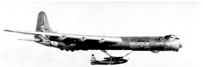
An F-84F hangs under a B-36 in its trapeze.
