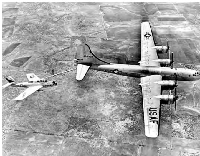
An early refueling operation, with a KB-29 supplying the fuel.
