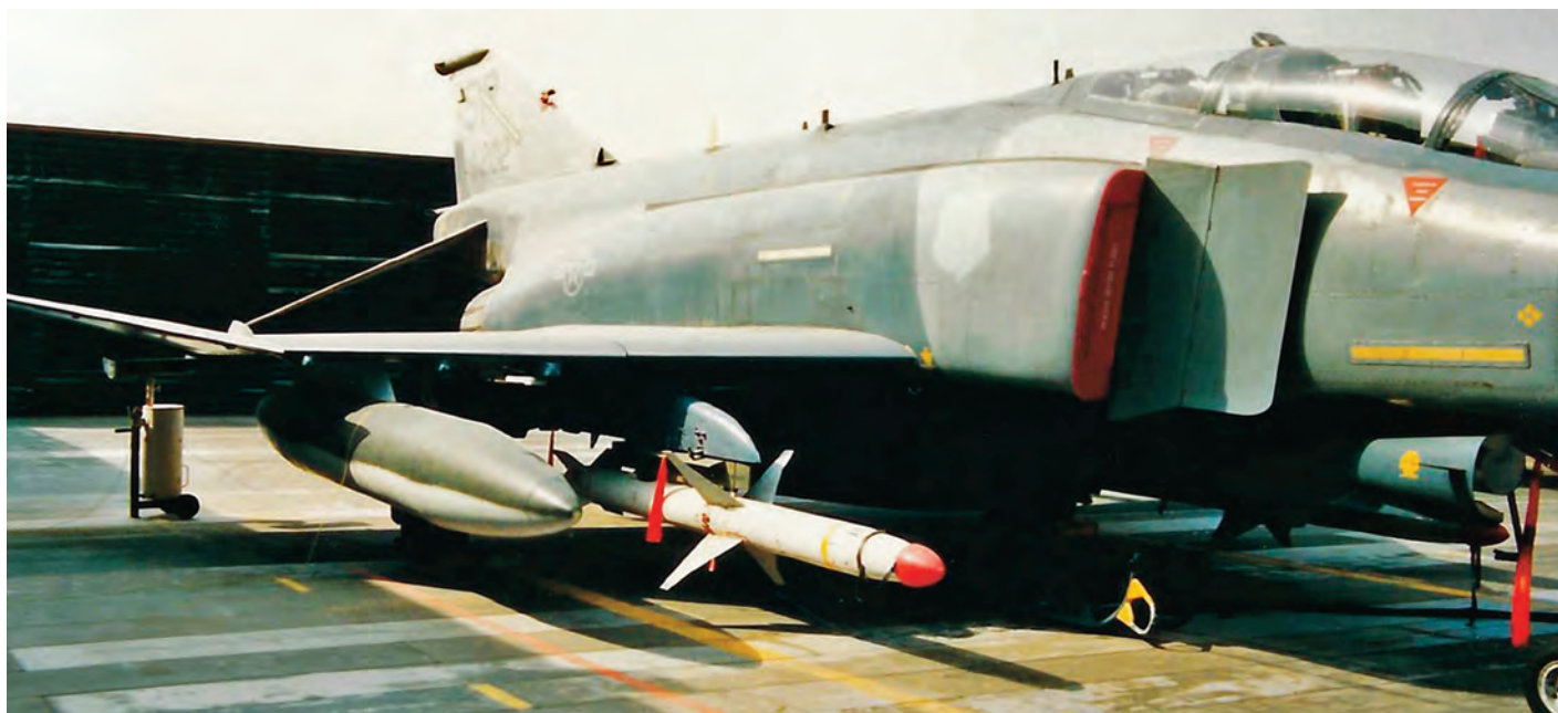
F-4G 69-7202 of the 81st TFS in its hard stand at Shaikh Isa. The Weasel is configured with two AGM-88s. The 52nd TFW patch was removed. (Victor Ballanco)
