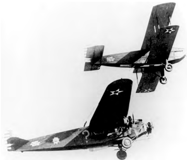
Atlantic C-2A (aka Fokker F.VII) Question Mark refueled by a Douglas C-1, in an early test of aerial refueling.
